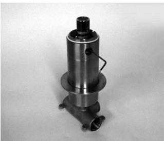
6. To access the internal mechanism, remove the casing.
