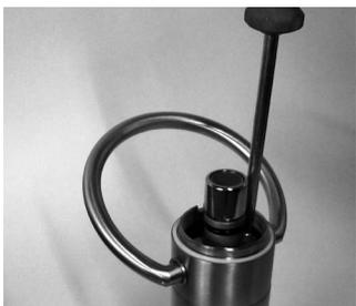
4. Loosen two screws so that the ring handle can be detached.
