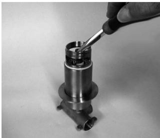
9. Using pliers, unscrew the inner ring from the cartridge, and then remove the cartridge.
