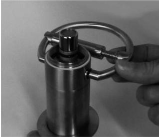
5. Remove the ring handle using the accessory provided and disassemble the faucet.
